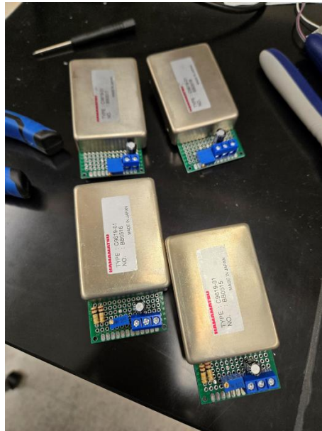
Fig. 5. Power supplies for modules 3 and 4 (for both the PMT and the MPPC).
