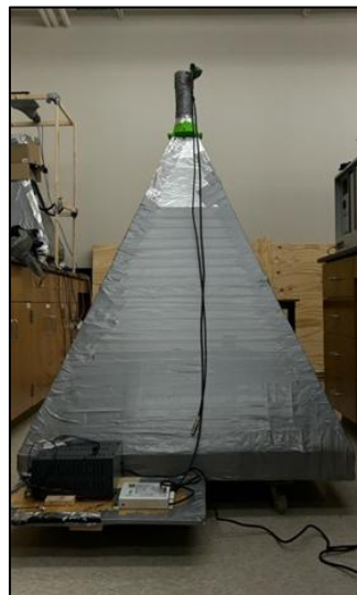
Fig. 3. Detector module 1. The 3D printed PMT holder is at the top, shown before covered by light-tight cover.
